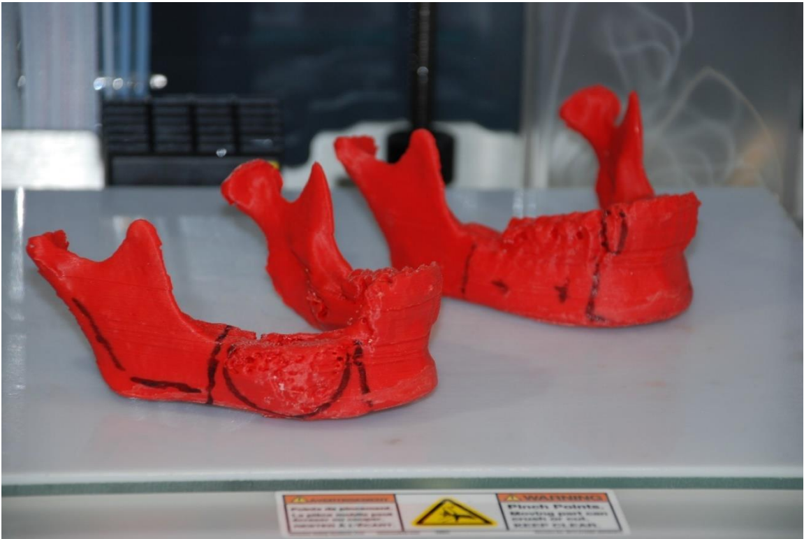
Figure 8. Bio-Models printed on 3D Systems CubePro Trios.
