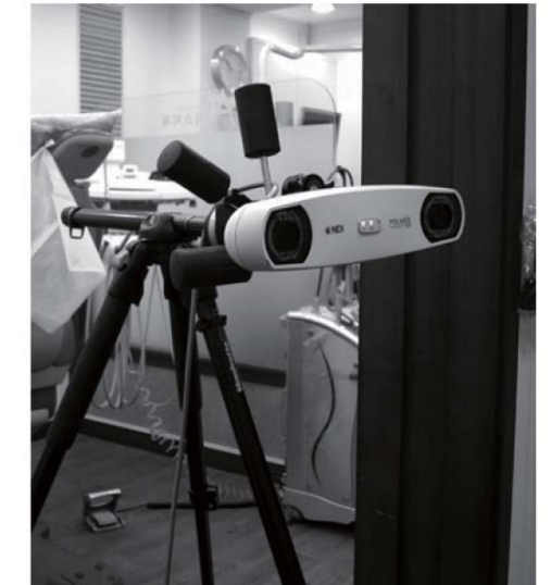
Fig 2. Optical tracker (Polaris Vicra System, Northern Digital, Waterloo, Canada).
